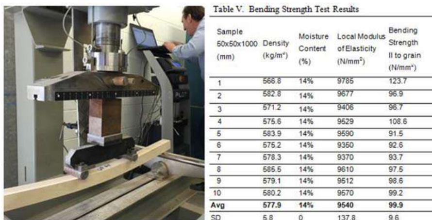
Figure 8: Bending strength test.
