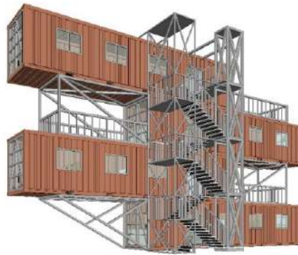
Figure 17: Combination form of container house.
