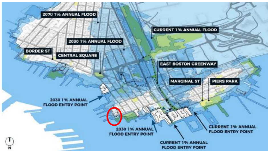
Figure 5: Sea level rise without intervention for a 100-year storm event in 2030 (9"/23 cm) and 2070 (36"/66 cm). (Source: www.boston.gov )
